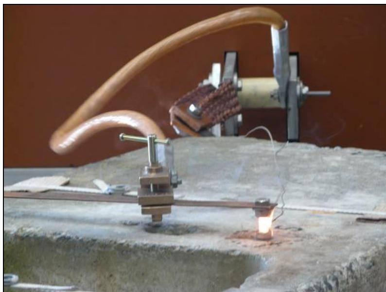
Figure 4: High current testing Vierendeel pole cage bond, with connection bolt white hot.
