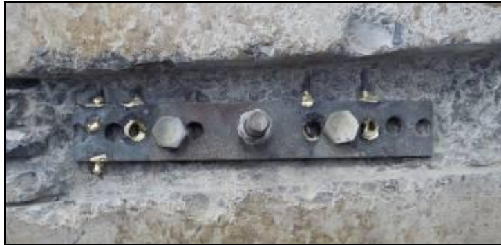
Figure 9: Design 1B- Test sample 1- Brazed bonding plate joint.
