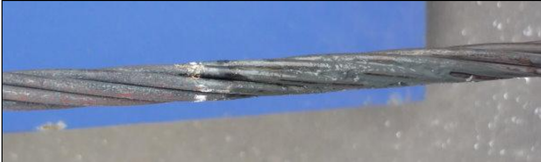
Figure 12: Strand removed from connection ferrule after high current test. The outer edge of the connector is shown by the white ring, the location of the first grub screw is in black and jointing compound in as-new condition can be seen beyond that.
